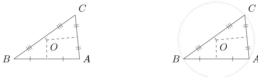
(a) Perpendicular bisectors of the sides. (b) The circle can then be drawn.
